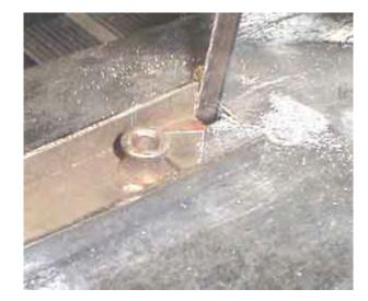
The trusty Jet Taiwan bandsaw comes into play again as we cut the triangle out, leaving the flange intact. You can barley see the first flange because it is reflecting the bandsaw surface but it's there.
