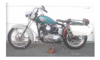
You can see the crash bar doesn't seem to match the bags on this side. Since the left and right mounts were bolted together and matched as they were made this means the problem is in the crash bar. I needs to be straightened out and the angle changed like on the right side one. One day, for now I need to go to Albertson's and buy groceries so I can try out my new bags. Later.
