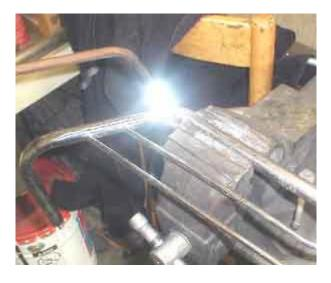
Here the trusty torch is used to heat up the corner of the bars so I can bend them a little so they match the angle of the bags. Bad move, it turns out, because someone had done the exact same thing previously. The bend had a crack in it that was filled with brazing. This melted out and left a big hole, but at least the bars were in the right position. This was important because I would use these bars as the template to make the mounts that will weld up to my cut-up struts.
