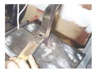
This is going to look so good. Better yet, the strut will give side to side structure which the bags need down low. Not only that but the big bike struts have a 3/8 hole in the end that is the exact size of the stud in the crash bars. Life is good. Here that howling sound? The big bike people crying. Ha ha, I laugh at their anguish. To get these bags mounted I would have cut a generator Shovelhead in half.
