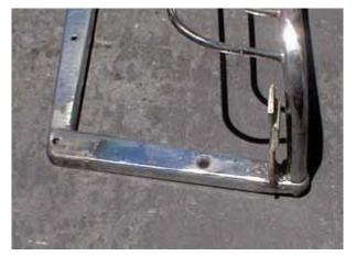
Here is the big-bike strut welded to the Sporty strut. I had to take this picture after the whole job was finished to replace a bad shot so you can see the little bracket already welded on to hold the bags at the bottom. Pretend it isn't there-- you are looking into the future.
