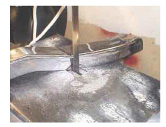
What about the front mount for the crash bars? Well, I had two little pieces of big bike strut left over and the flatter part on the far side of the bandsaw blade looked perfect for the job.
