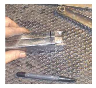
I do remember this part. This is where I convinced myself the flanges were too long for the angle they were supposed to mate at. Here I am holding both the left and right bigbike struts marked for trimming. At the bottom picture you can see the huge gap just about this long. I do need to make that board longer after all.
