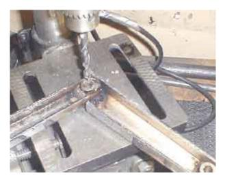
Before I could evaluate if the length and angle were correct I had to drill the flange of the big-bike strut where it covered the hole in the sporty strut. The sporty strut is the perfect pilot for the 5/16 drill.
