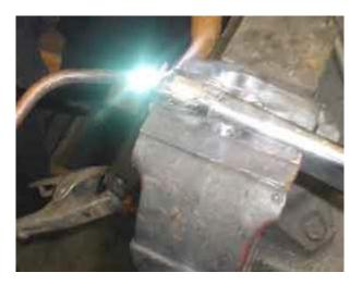
All my fretting must have paid off because the strut lined up perfectly. Here I am welding up all the places where I can join the two struts. You can see the arc welder ground clamp in the background. I arc welded most of the joints. I used the torch to weld the flanges up all nice and pretty. When sanded on the belt sander it looks like one part. Of course I used this part as a template for the left hand mount. I just bolted the left and right struts together and welded away.
