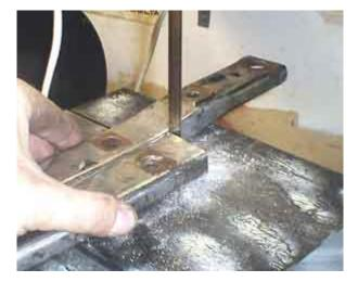
Same as with the bags, it's easier to make the other side at the same time. Using the first one as a measuring stick I cut the second one to the identical length. Note the rust and chrome peeling around bolt holes. This is a perfect use for these bars-- they aren't pretty enough to run but no one will see the rust where I will mount them.
