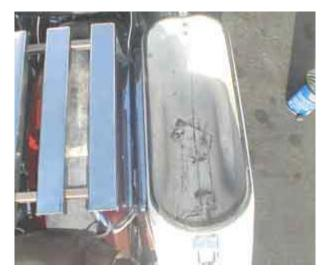
The bag is mounted with the cut up strut in position. The luggage rack is sandwiched between the struts and bag is far enough out to miss the chain-gaurd (it's really the break lever that's closest). The greatest thing about this is how the cut-up strut fills the gap and makes the installation more integrated. I am pointing the nice face of the cut strut inward but I will be changing that in a few pictures. Stay tuned.
