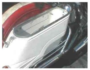
Here we see the bag mounted with it's new holes. I checked out that there would be room for the crash bag between the shock and the bag and that the chain-gaurd would clear the bag even when the swing arm was fully up from a heavy load or a big bump. You can see the front bolt misses the reinforcing plate but we'll fix that in a bit.
