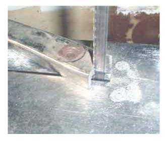
This picture shows the other side of the semicircle being cut out. It looks like the bandsaw blade is casting a shadow across the strut bit really that's the hole from where we cut out the first little triangle.
