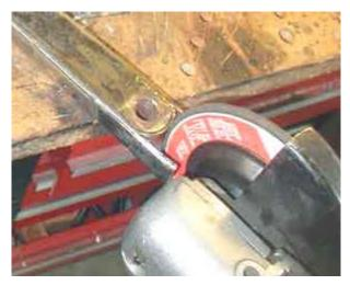
The right-angle grinder takes off the last bit of metal to get a perfect semicircle. The bandsaw was especially useful to cut right down to where the semicircle meets the side flange. Po folk can use a file. Don't despair, it builds character and creates the lust for power tools that makes you a good American..
