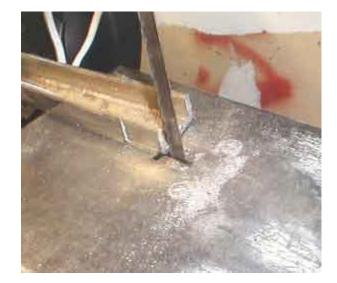
OK, cut the flange off where the other strut will mate to it.
