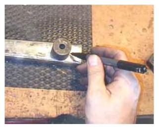
Now for the nice touch and the explanation of why I cut the struts longer then needed. I found a big spacer about the right size to draw a semicircle around the forward bolt hole. This is the nice round shape I want the strut to have in the front.
