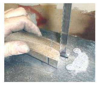
Because this flange is wide I decided to cut the flanges short and bend the main web over to cap off the end.
