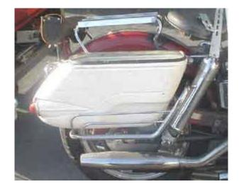
Here's the bag from the side. It bugs me that the crash bar angle does not match up with the angle of the bags so....
