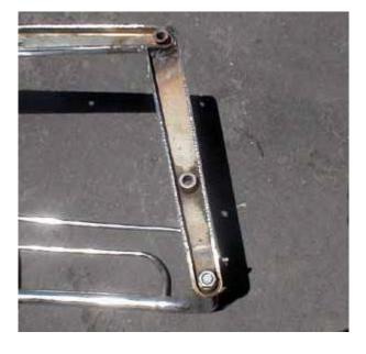
A rear view of the big-bike strut welded to the sporty strut. A little weld spatter but that automatic helmet that darkens when you strike the arc makes it a lot easier to weld. Those auto-darkening helmets were invented for fighter jet pilots so they would not be blinded by nuclear blasts. The cold war making your welding tasks easier. I love it.
