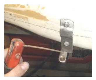
The last thing was to weld up was the little bracket that holds the bags at the bottom. It had a right angle bend on it that I cut off at the right length to space the bag away from the mount. I first just marked this part and tried to weld it without the bag on. Duh. I then cut it off and used the bag as a template to position it. It has to line up perfectly now. Tack it on with the bag in place and then pull the bag and weld it up nice on both sides.
