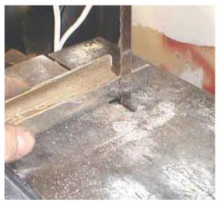
There was a ton of eyeballin' and cogitatin' and calculatin' to get the length of the strut right. Here I am cutting off the flange where this strut will mate to the first struts I built. I hope your dad told you the carpenter's motto: "Measure twice, cut once, you can't make a board longer." Fortunately we can weld a strut longer but why do it when it only makes the po' folk cry with envy?
