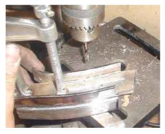
A lot more cogitatin' and measuring and I drill the hole to mount the front mount of the crash bars. You can see the flanges on the left splayed out and ready to weld to the sporty strut. The existing hole in the big bike strut was almost cut in half when we made the other piece that mounts the bags at the rear, but this partial hole lines up with the front mounting hole of the sportster strut. Once again, the welds can break and the part will still be attached.
