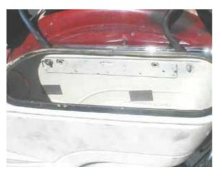
Now you can put the bags into place and work the long bolts through the mounting holes. The bags are already screwed to the little bracket at the bottom. It's a little difficult but you can just get your hand behind the shock and fender to push the front bolt through. It's a little easier to run your hand up the tire from behind to push the rear bolt through.
