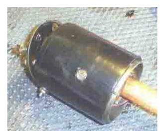
It's usually easier to put the brush plate on after the frame is installed. This plate was too snug to pop out so the handle of the mallet was used to gently tap it free. You can leave the wire attached but don't get too rude with it. I also was using paper towels to dry off any oil on the parts.
