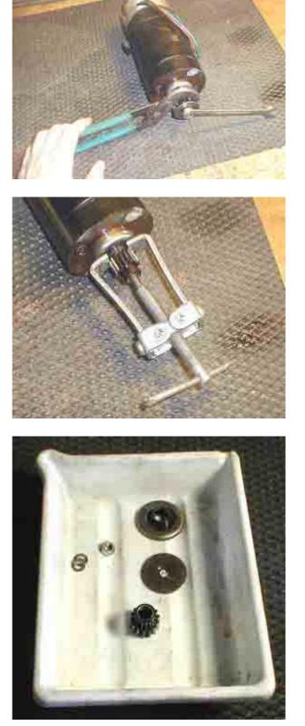
It's scary putting channel locks on a gear but that's the only way I have been able to do it all these years. Nut is conventional right hand thread.
