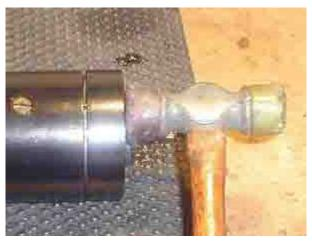
The frame didn't want to slip on so I pulled it from the vise and after cleaning the pin and hole, I gently tapped the end bell on with a small rubber mallet.
