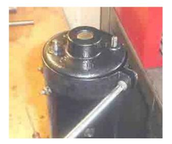
Since the voltage regulator uses the generator bolts I loose assembled the brush cover. I used to run without the cover to let cool air into the generator. It worked great in the rain, everywhere for 5 years. Until I blew a front fork seal and the fork oil splashed on the commutator. It glazed it over and ruined the voltage regulator. I went back to running the cover.
