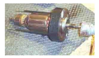
Gently tap armature out off the end bell with a small rubber mallet. I really mean rubber-- if you use a regular hammer you will mash the threads on the and and life will be difficult. If you must be a wino at least thread the nut back on the armature and pound on the nut.
