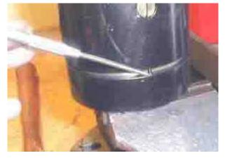
Note the little pin in the frame and the hole in the gear side end bell. It can only go together one way.
