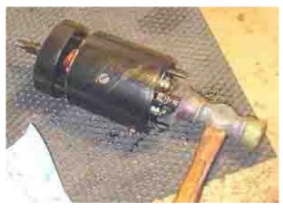
To get the armature out of the frame you can gently tap on the armature with a small rubber mallet..
