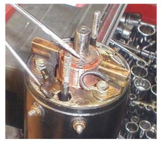
One wire is rubbing against the commutator and the other will get pinched by the end-bell. Bend them back out of the way or loosen and re-tighten the terminal to keep them out of harm's way.
