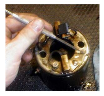
Note the little pin in the frame and the little slot in the brush plate. It has to go together one way only.
