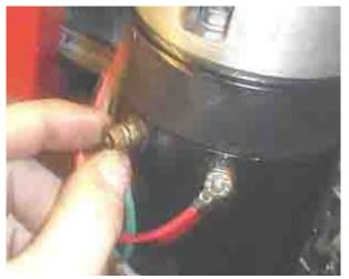
For this setup that uses a Franks electric regulator you can hook the field and armature wires up now. Check your notes and you do have the original instructions on file don't you? Don't trust the color on these wires. Different regulators have different colors. Note the little internal tooth star lockwashers that insure good electrical contact. The hardware store is your friend. Spend time with your friends.
