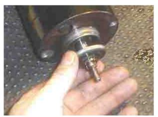
Make sure everything is spotlessly clean and especially this bearing cover. Dirt and grime in a precision ball bearing is not good.
