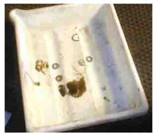
See why professionals use the trays? The only things left over are the 3 lockwashers that were replaced with new ones. One for the armature nut, two others for the end bell studs.
