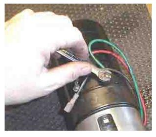
This particular generator has a Frank's voltage regulator mounted on it. A 3/8 inch wrench or nut driver will remove the field and armature wires. Jot down the colors if you aren't sure of how they go. There is an "A" and an "F" stamped in the generator next to the terminals to identify them.
