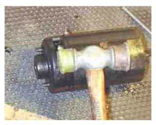
Gently tap end bell off by lightly tapping under the cutouts with a small rubber mallet. Alternate tapping on both sides to insure nothing gets bent.
