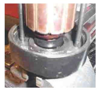
We finally get to see the problem: When the old '62 sat for a month the motor sumped. This means the oil in the oil tank leaked down into the motor. When I started it all the oil was forced into the gearcase. A bunch of oil blew out the gearcase breather tube but the pressure got high enough to push this oil seal out of the generator. Oil leaked out the generator every time I ran the bike since.
