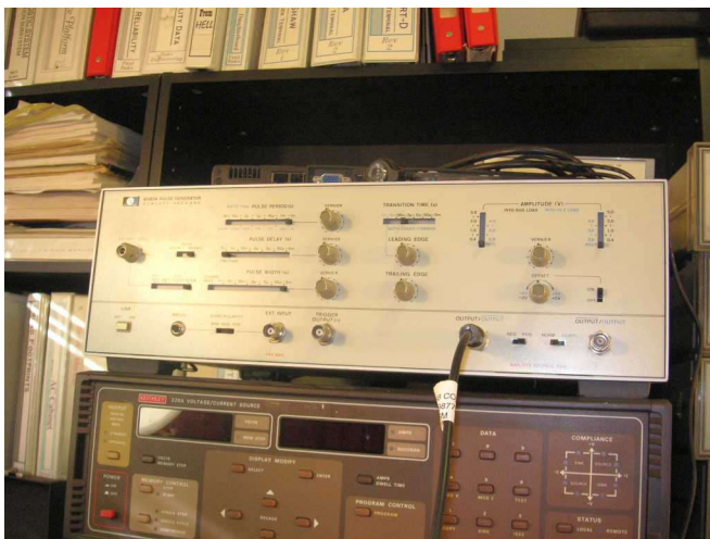
This HP 8082A pulse generator feeds the Picosecond pulse generator.
