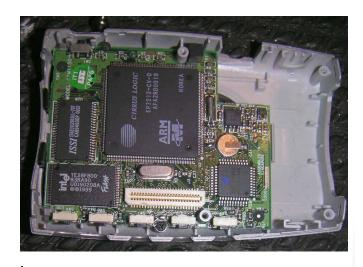
You can see the top case half here. That ARM-core microcontroller, and an Intel flash memory, I assume for settings.
