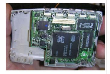
Here you can see a third crystal, the round watch crystal to the left of the ARM chip. There is also a tiny lithium battery, perhaps to save settings when changing batteries. Not sure why they needed flash memory and a hold-up battery both.
