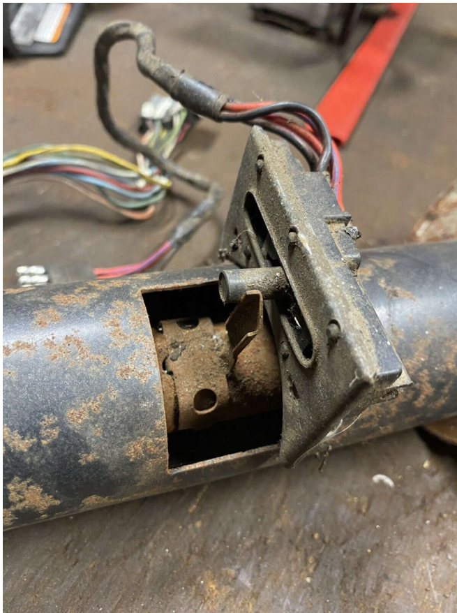
This is the reverse switch on the column.
