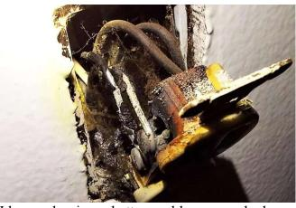
I knew aluminum battery cables were a bad idea because I knew how many fires aluminum wire caused in houses. It was considered a serious fire hazard even back in 1980. Today the code still allows aluminum house wiring, but electricians are instructed to use an anti-corrosive coating, and to to torque the terminal to a very specific tight tolerance.
