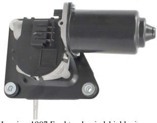
Here is a 1987 Ford truck windshield wiper motor. They had gone back to the worm-gear design. The precise die casting that locates the motor and worm gear also locates the driven gear. That, plus the fact it is not a spur gear train, make the motor strong, quiet, and dependable.
