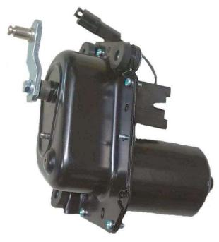
Here is the 1980 Ford truck wiper motor. It started off with all plastic gears. Those broke in testing, so they had to make a few gears out of metal, so now the cost savings was a penalty. Once we got it in a prototype cab, the noise problem appeared.
