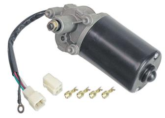
The 1979 design worked fine, but did have several problems. The "pigtail" wires coming out of it were used by assembly workers to carry 5 or 6 motors when they got behind on the line. The loose connector also had to be restrained so that it did not rattle when you were on rough roads. There was also a ring terminal needed for a ground. The 1980 design had a direct connection and no ground wire.
