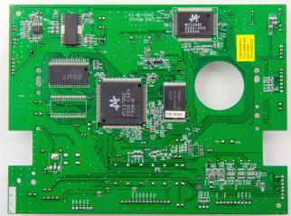
I said no problem, just replace it with an FR-4 board. That is a fiberglass epoxy construction. FR does not mean fiberglass reinforced, it means "flame resistant". With no paper content, these boards would not burn, but they were also much stronger.
