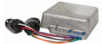
In addition to the packaging in the engine compartment, the module also had pigtails, something discussed in our wiper motor disaster article. It was the same problem. Assembly workers could carry six or eight modules by the wire pigtails. This would break the wires and cause failure at the end of the assembly line. The wire pigtails also had a rattle problem. You have to secure those connectors so they don't make noise when you drive over rough roads.
