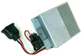
This is another aftermarket ignition module. They put fins where the high-current transistors are, and left the module smooth elsewhere. Pretty smart. When under the hood, the fins transfers heat out, but the cooler part of the module is smooth, minimizing heat transfer in.
