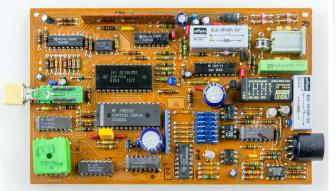
This is an example of a paper-phenolic circuit board. It is made from layers of paper glued together with thermoset phenolic plastic. You can often see them inside appliances and older cheap consumer electronics.
