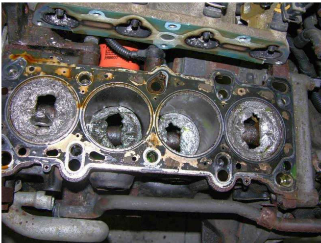
Figure 2; After his timing belt broke, Mike Robins (tinman19672009) can confirm his 2002 Kia Rio has an interfering engine.
