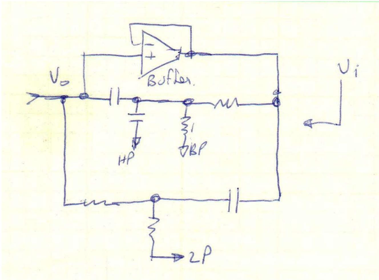
Application engineer Mike Wurtz showed me this simple multi-output filter circuit. It uses one op amp and yields high-pass, low-pass, and band-pass filter functions. Lede col 2.
