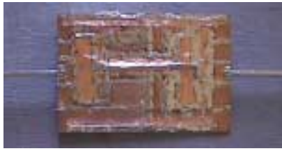
Figure 5 This copper-clad board has two antennas soldered to opposite sides of the same ground plane. When you operate circuits with fast edges on the board, the antennas radiate significant amounts of RF, even though they galvanically connect (courtesy Glen Dash).
