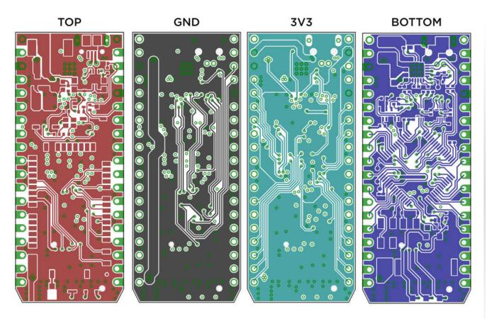
I asked Oscar at Proto Express what files they need to fabricate a circuit board. He sent the following list. While I usually don't send the assembly drawing, I always make a fab drawing so the specifications are clear.
