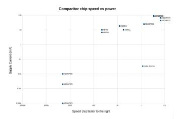
This chart shows Analog Devices comparators. You can see ADI has the fastest chip, and that that speed requires a significant amount of power. You can also note they don't offer dozens of chips, just ones targeted for specific applications.
