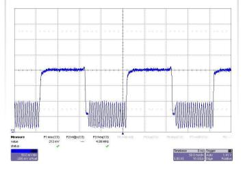
Figure 1 might make the problem more understandable. The rising edge of the pulse is probably what you will trigger off of. The little 600 MHz oscillation on top of the pulse is asynchronous to the big pulse. It comes from a free-running oscillator that has nothing to do
