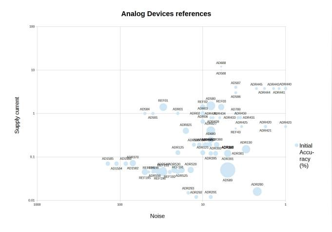
Here is a spreadsheet I did about Analog Devices comparator chips. The spreadsheet has selection filters that can help you narrow down the part you need. The chart above from that spreadsheet shows the tradeoff between noise and power consumption. A circuit that uses higher current tends to have lower noise. An added feature of the chart is the bubble size that shows initial accurate, another critical spec for voltage references.
