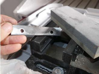
I used a sharpening stone to flatten the back side of the fixed jaw.
