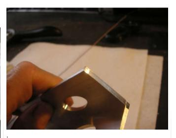
The part measured much longer than design intent, 5.020 on the left flange. You can see the divot in the end of the flange where the end mill ran off the part. Measuring to this depression made a slightly better 5.008 length.
