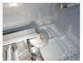
This uncovered the fact that I had a 0.100" error in the part zero origin in SolidWorks CAM. The two sides were exactly 0.1" off. I corrected this for the next run, and I plan on using the same speeds and feeds as in this run, only to remember to turn on the dang Micro-drop coolant, so the end mill does not load up. Thankfully, I received two square-nose end mills from avid when I ordered the mill.
