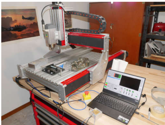
The Avid Benchtop Pro is a router-style mill.
