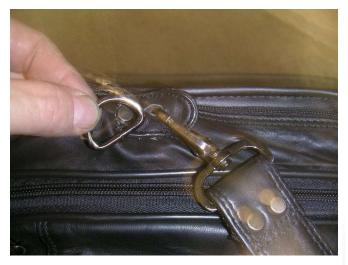
Here you can see where the D\_ring tore out of the leather. I poked a hole in the leather tab and hooked the strap clip into that hole as a field expedient.
