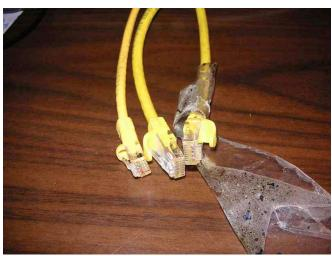
Here is the CAT-5 cable with the broken tab on the right. You can see the grungy tape that I tried to use to hold the connector into the printer. I suffered with this kludge for years.
