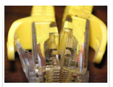
Here is a close-up of the CAT-5 connector with the broken tab, on the right. The other end is on the left, it worked just dandy on the hub. Yeah, I considered just reversing the cable and using the good side on the printer, but I knew it was inevitable the broken connector would just pop out of the hub one day, to re-incense me. I also considered borrowing a crimper to replace the broken connector.
