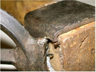
It looks to be a classic fatigue crack from thin metal of poor quality.
