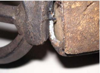
You can see the older rusted crack and then the fresh metal crack where it just gave out.
