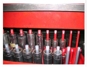
Here you can see the how the pins on the 3/8" drive deep-wells just clears the depth of the drawer. Problem is that the 1/2" drive deep-well pins on the other tray are way too long to fit in the drawer upright.
