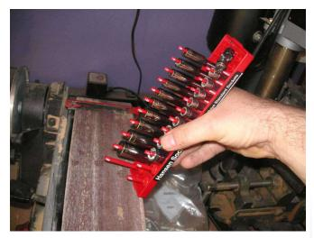
I also had to grind the little tabs down on the side of two trays so the would fit in my particular toolbox drawer.
