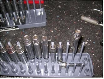
The first problem I had with the Hansen socket rack was that my Snap-On 1/4" drive metric sockets did not all fit on the pins. The center hole in these four sockets are smaller than the plastic pin.
