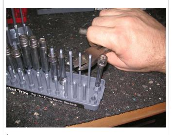
ECO (engineering change order) approved, as we say in the design community. I just cut the pins shorter with a pair of Dykes. Drills don't cut the hardened steel sockets. The pins are still long enough to keep the socket from falling over. I can't say the same about the little pin on the far right meant to hold the 4mm deep-well. I may have to re-engineer that with a deeper tube or a metal screw from underneath instead of the short plastic pin.
