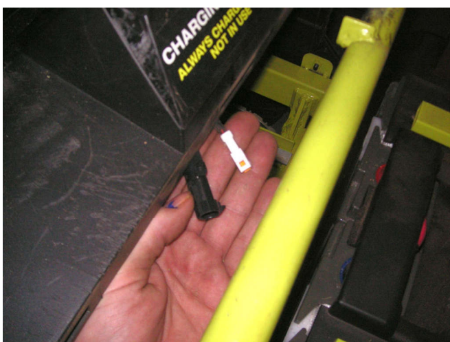
The charge port has a black connector for cutout sensing, a white one for the thermistor.
