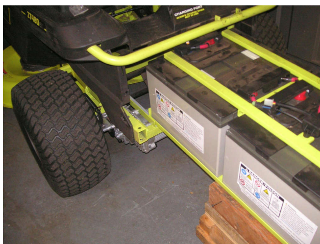
I picked the tray up and started in the slides. Be sure to clean so the tray slides all the way in.
