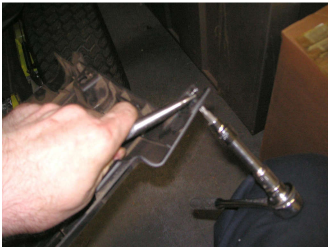
Rear cover misery. I get the two J-nuts off. They just ripped out the thin plastic.
