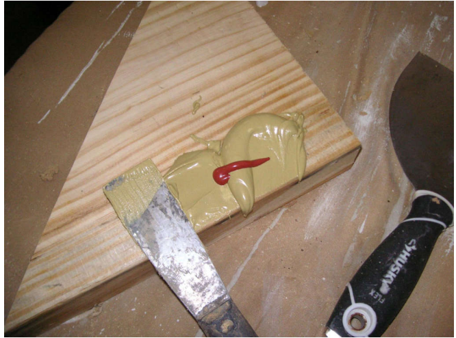
Too much hardener, froze up in two minutes. Hole in hardener tube should be 2mm wide.
