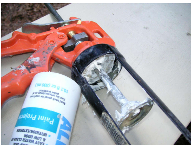
I bought 5 tubes of caulk and used them all on the three walls. This old tube blew backwards.
