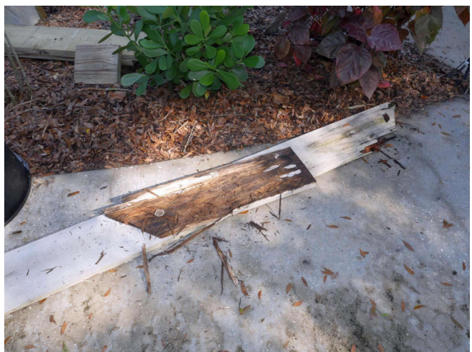
The short top piece is rotted at both ends. Using the pressure-treated wood solves this.
