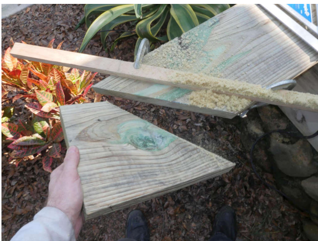
Go slow and support the cut piece and it will give a nice accurate 45-degree cut.
