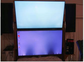
Here is the dying Sharp. I had turned up the brightness to use as a monitor, the LEDs died.
