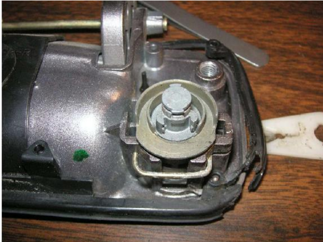
The back of the key tumbler where the lever attaches.
