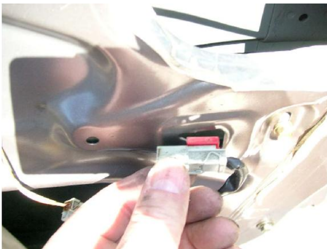
The connector slides onto the tang in the door. Honda does a great job making sure there are no rattles in the door. Nothing is left to flop around. I hope the new ones are this good.
