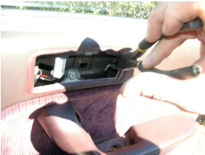
You have to pry the handle rod forward to get it on the handle. Nowhere in the manual does it make clear that you pull the whole handle forward to get it out or in, it has little tanks.
