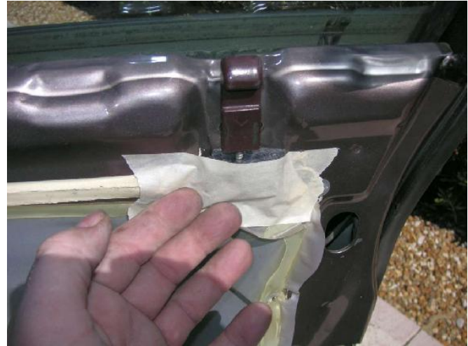
The plastic rain liner tore and the dum-dum is not sticky, so a little masking tape serves.
