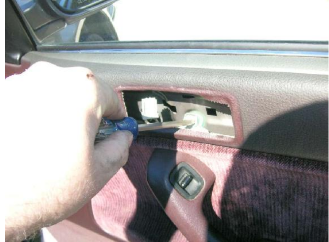
A screw that goes under the door handle.
