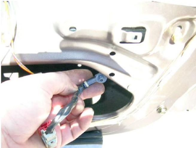
The wire harness has a clip on the inside.
