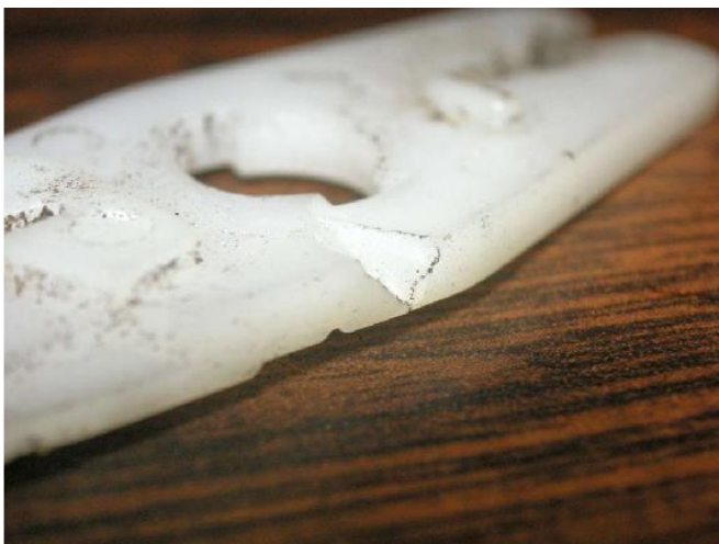
Another close-up of the cracked lever. What an immense pain to replace this mess.
