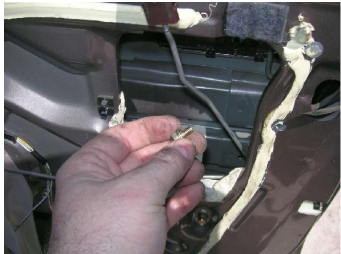
The two screws for the door handle.
