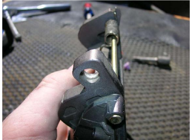
Now the door handle goes back in. It had a gasket that was torn a bit but it was good enough to go back in.
