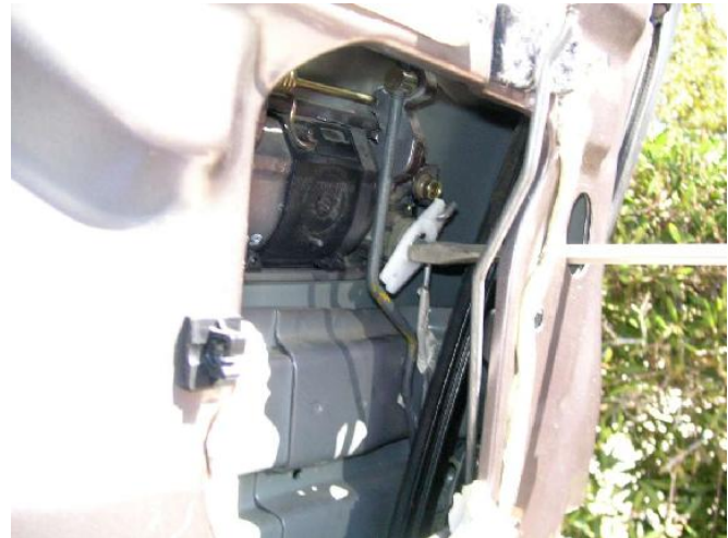
Photo of Middle Inside Left Front Door of 1994 Accord Showing Key-Driven and Handle-Driven Mechanical Lock and Latch Actuator Assemblies
