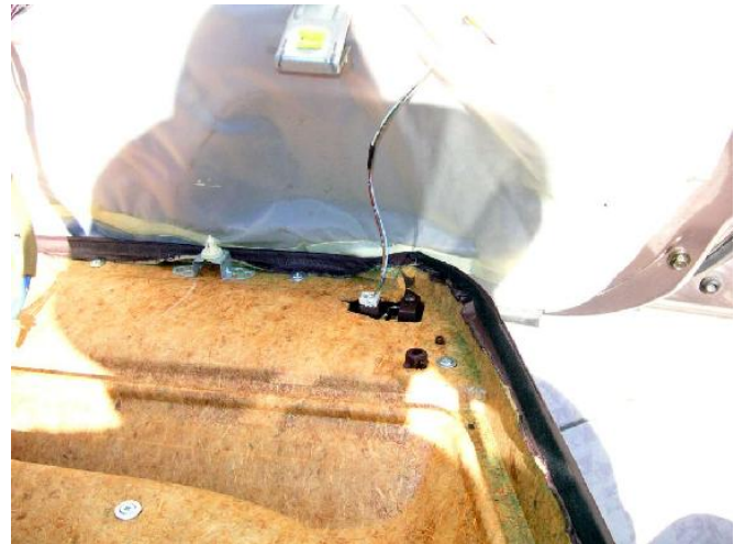
There is a little running light that you hook up at the bottom of the inside door panel.
