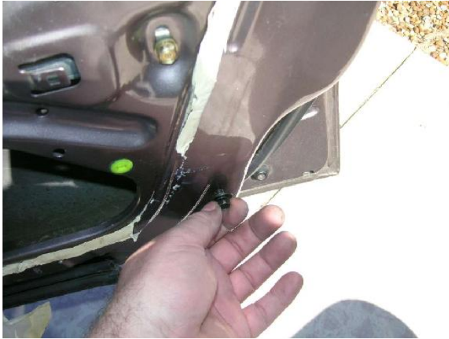
The bolt for the window track goes back in.
