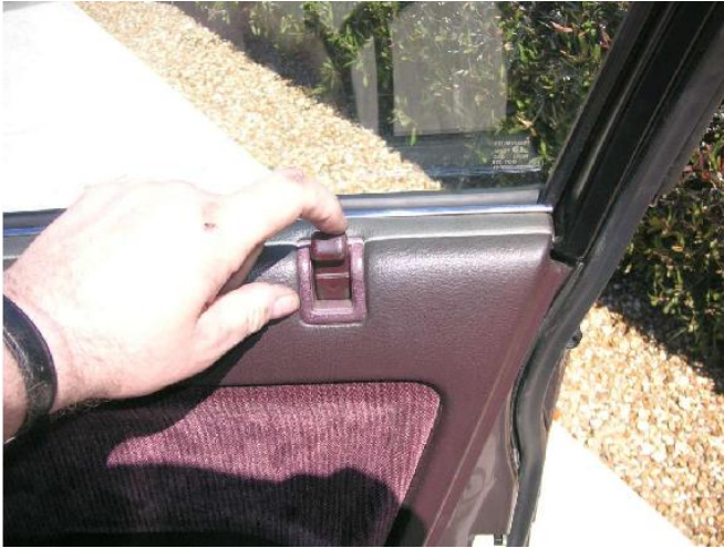
Verifying the lock button works, and the key. This unscrews to get the latch out, be sure to put in back on before you hang the door.
