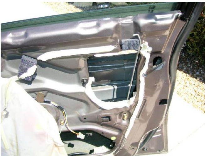
I taped two rods together to get them up the handle, while pulling the inside handle latch out the right hole. This was a horrid job.
