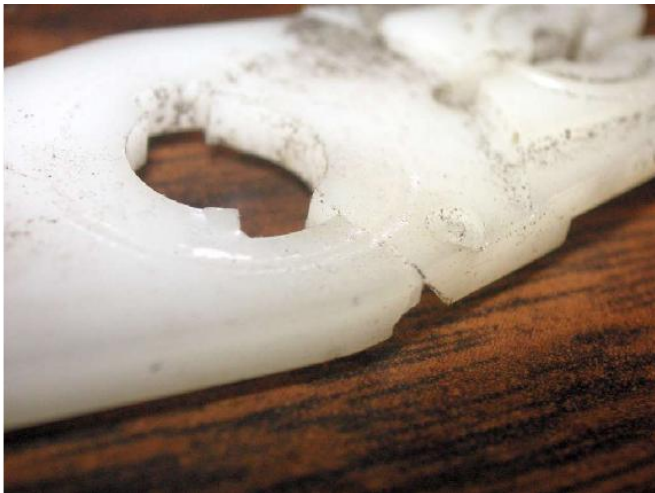
Here is a better close-up of the crack in the lever. The material looks to be nylon.
