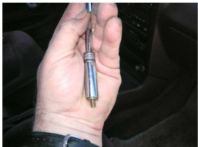
A deep-well 10mm socket lets you get the two door handle screws installed from the inside.
