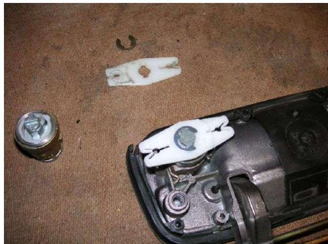
The new cir-clip seemed to work better than the factory one. I made sure the lever was not on backwards like happened at the factory.
