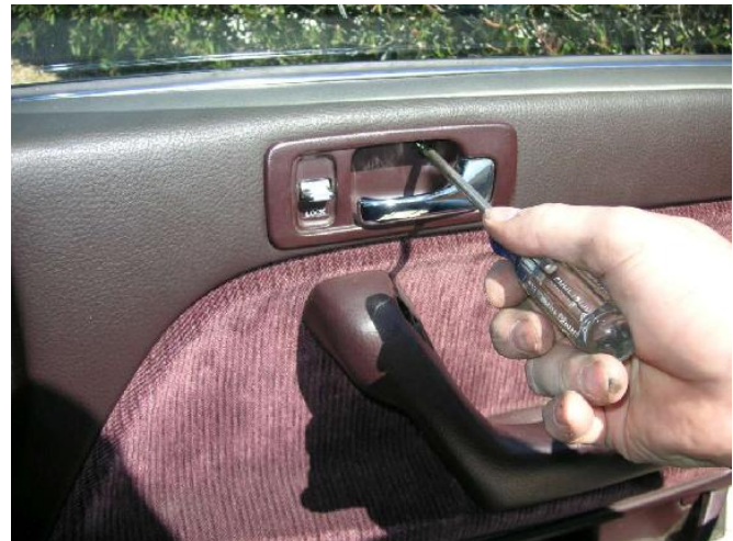
One last screw holds the inside door handle in. It had a cap but it broke up when I removed it. The handle does not flop out when you take the screw out, you have to pull it forward first.
