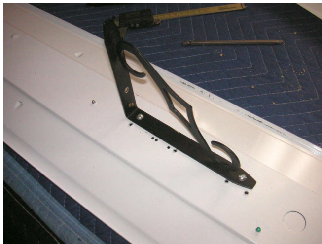
The same shelf brackets on the dual fixture works to mount the single fixture to the tripod.
