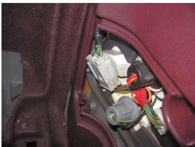
The harness connector clips to the body.
