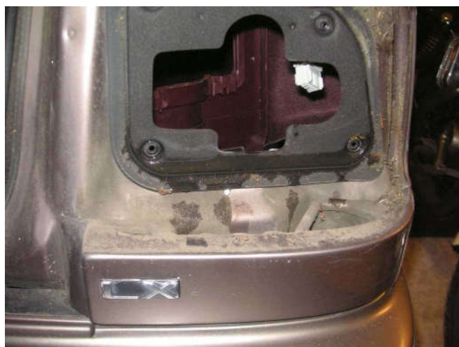
Water collected on the bottom but the leak is at the top on the other side of the gasket.
