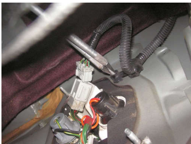
Here I use two X-acto knives to try and release the little tabs pressing against the stud. This is one of the little evils-- one-way clips.
