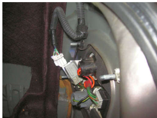
Now you have access to all 4 nuts holding the tail lamp housing.
