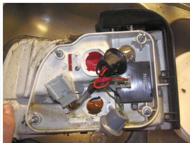
Backside of the right lamp, bulbs pulled.
