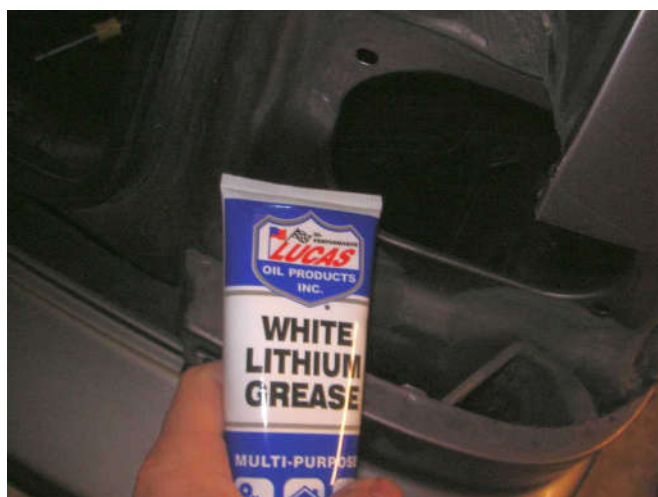
Rather than glue, I decided to use grease, to make it easy to take off, while repelling H 2 O.
