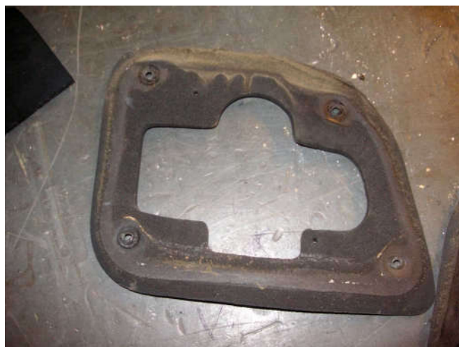
All this for this stupid leak. I might have saved this old gasket with the grease trick, but better to use new factory gaskets and be done with it. I don't want to do this job ever again.
