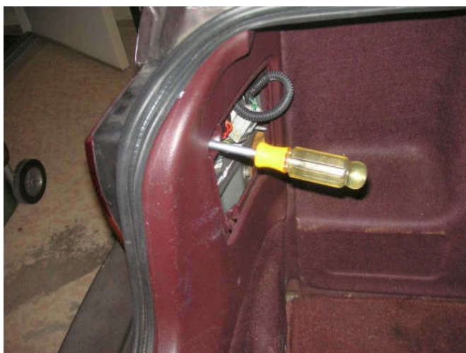
That fifth nut holds in the interior plastic.
