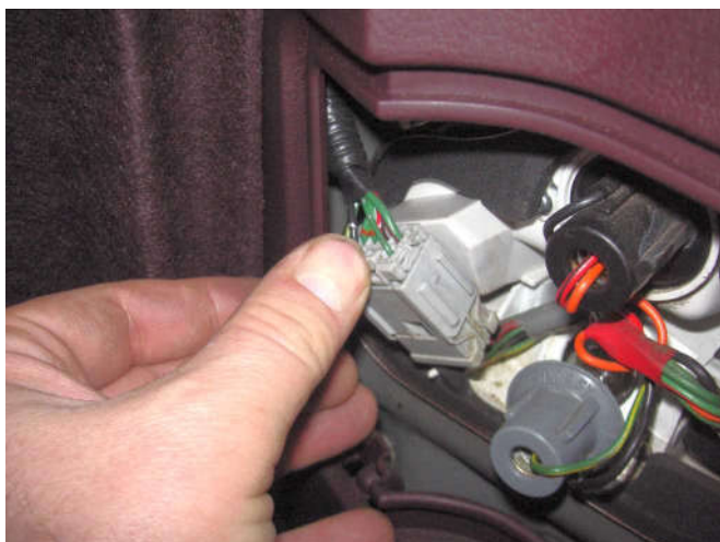
Satanic engineers dreamed up this release method. Press in on this little nub and it allows you to separate the connector.
