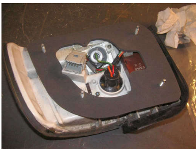
New gasket fitted to other lamp, bulbs in, and ready to go.
