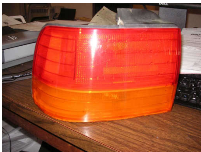
You can see about a half-inch of water inside the tail light, behind the orange plastic.
