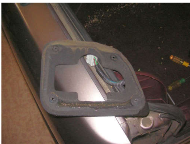
The front of the gasket show the drips.
