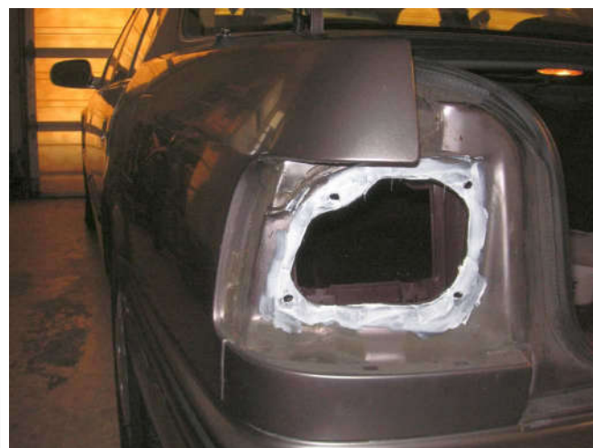
The left side cleaned and greased.
