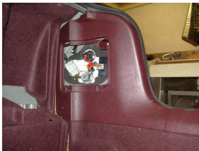
Popping off this inside cover provides access the bulbs but not all the screws.
