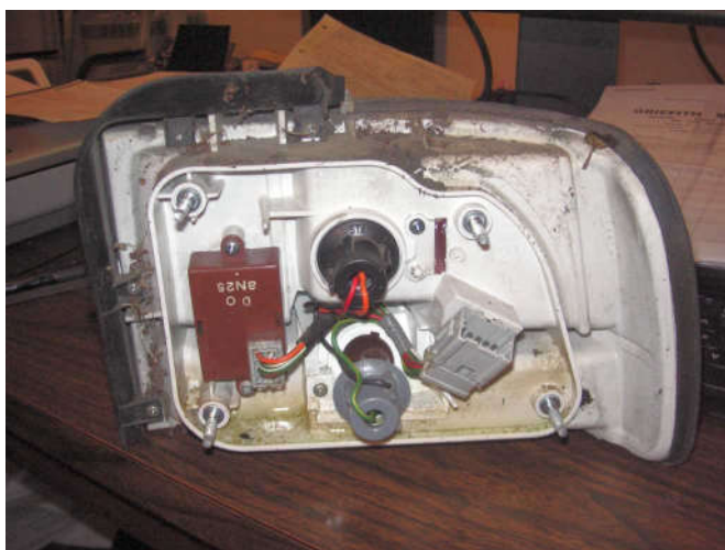
Here is the backside of the right tail light. The lip pressed against the gasket and seemed to seal OK on this side.
