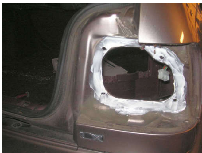
All greased up and ready for the lamp. The nice thing is I can take the lamp off without ruining the gasket, like with glue.
