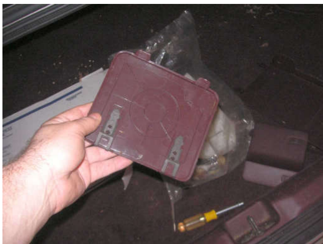
The covers over the lamp can be replaced, the little sliders are pretty straight-forward.
