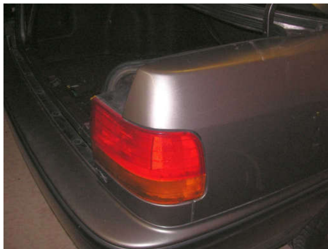
The right tail light has water and mold.
