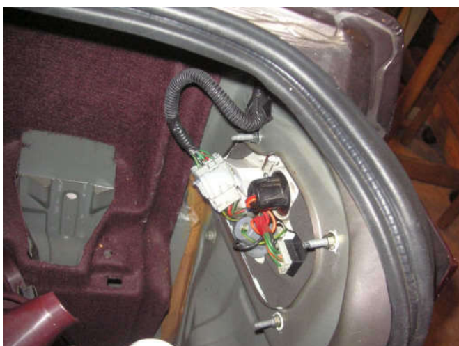
Harness connected, you can see how far back I had to pull the interior plastic to work on this.
