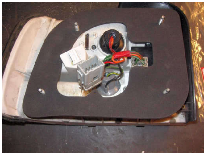
Bulbs back in, I had to clean a couple of the bulb contacts, a shot of DeOxit is a good idea.
