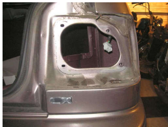
Right side has no rust, a good sealing surface.
