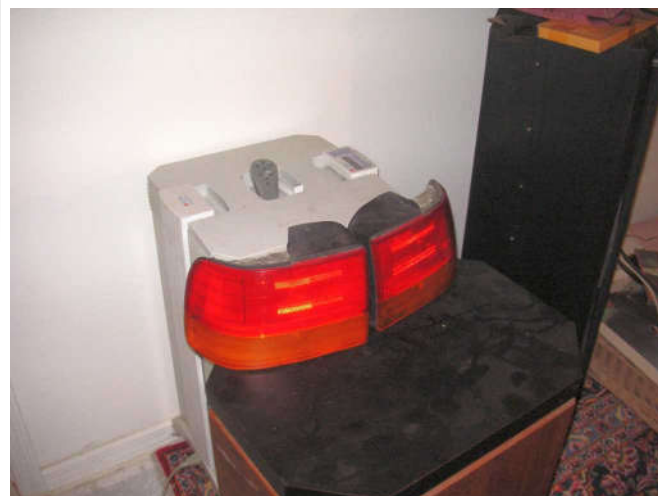
I drained the lamps and set them in front of my IQair HEPA filter for a couple days to dry them out. I also set them out in the sun.
