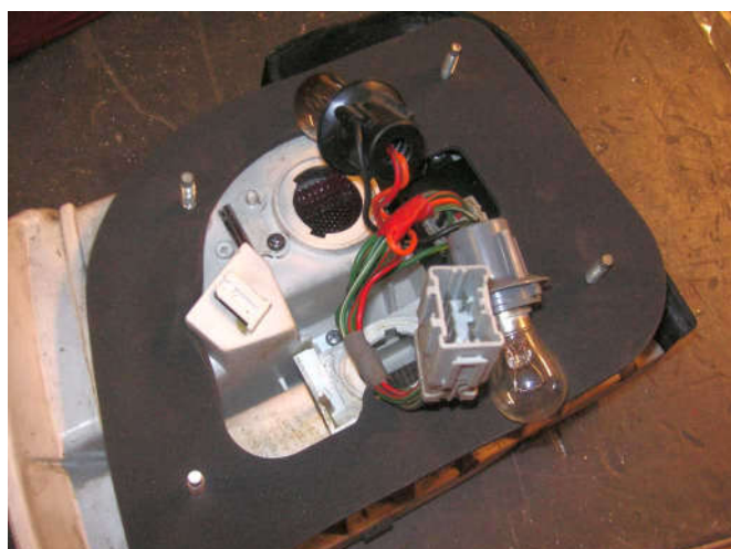
Gasket fitted to the tail lamp.
