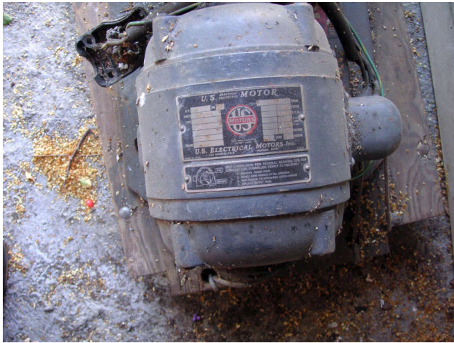
Here is the faceplate on the vacuum pump, It had a 3-phase motor.
