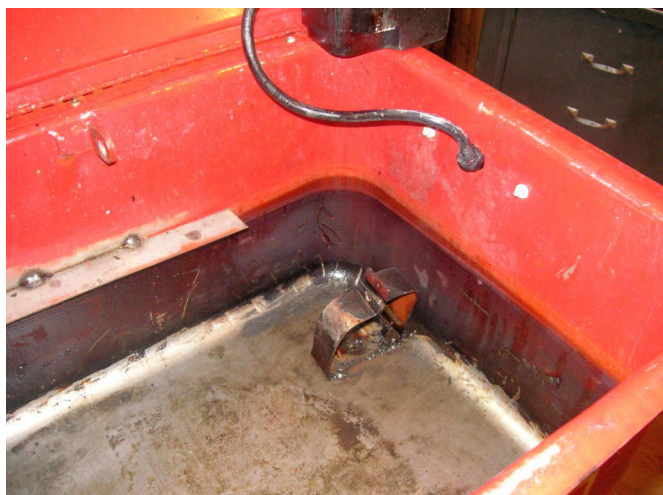
I re-mounted the pump, hoping to get it working one day, but it never unstuck.
