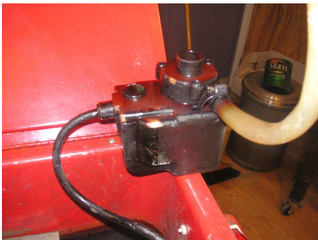
The pump got jammed. I never could get it freed up, I bought a new parts washer.
