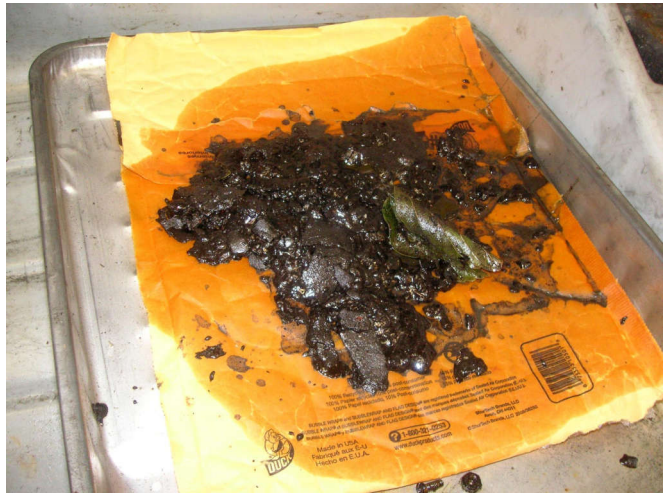
This is what came out of the parts washer. Putty knives and some steel wool did the trick.
