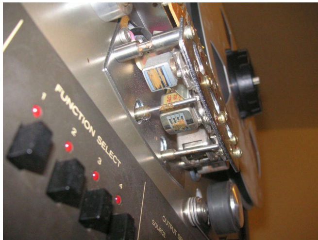
The heads got all gummed up. Denatured alcohol and a Q-tip got this cleaned off.
