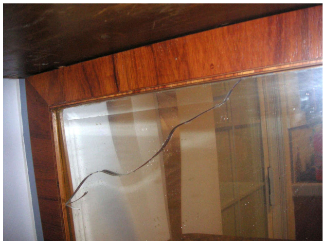
This crack in the beveled mirror was from me letting a popcorn popper get too close.
