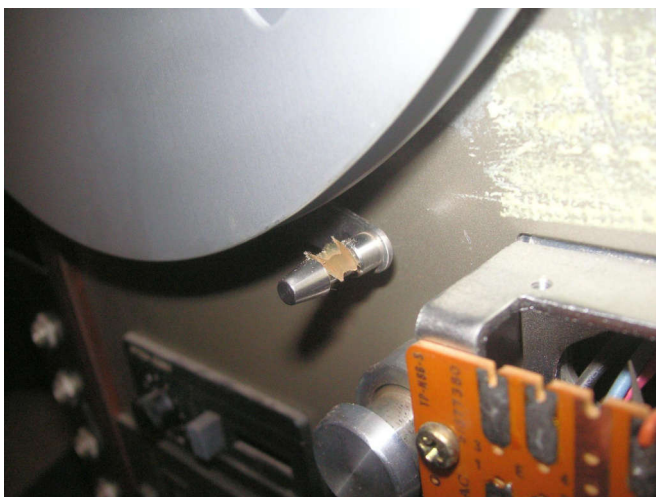
Even this good tape shed a ton of particles when I ran it though the machine.
