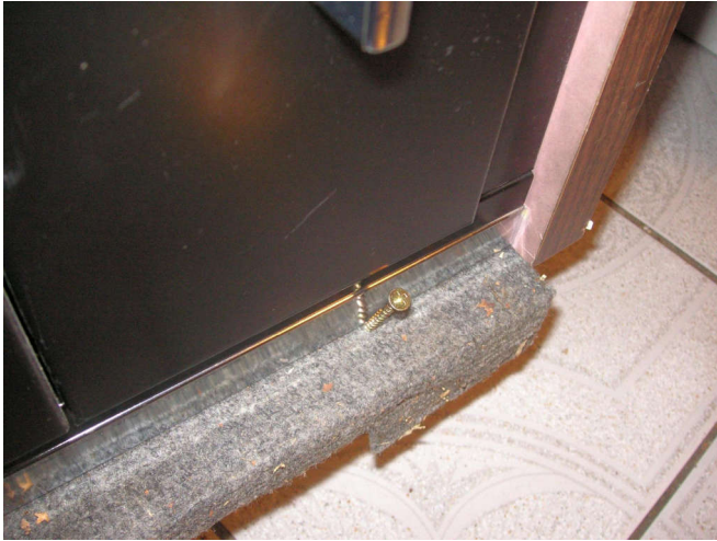
I learned to run a few construction screws into the dolly to keep the desk in place.
