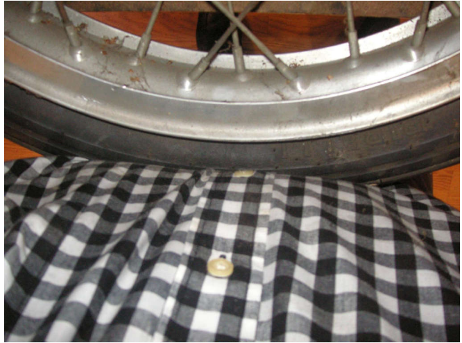
The trick is to use your belly to push the bottom of the tire into the recessed rim, spoons then can pry the other side up and over the rim.
