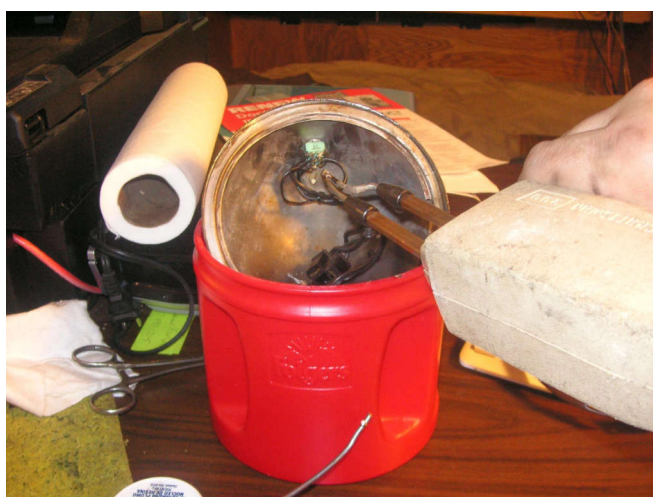
I put the high-beam switch in the Bates-style headlight. I needed to fix the wires.
