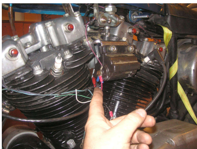
I get the electronic ignition hooked up. It might not be smart, a Dyna ignition may have been what burned the piston. Not enough advance.
