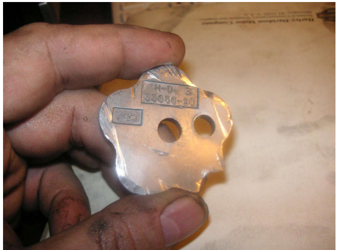
Here is the shifter detent drum, a little torn up from rubbing on the back of the clutch basket. Tomorrow I put it back together.
