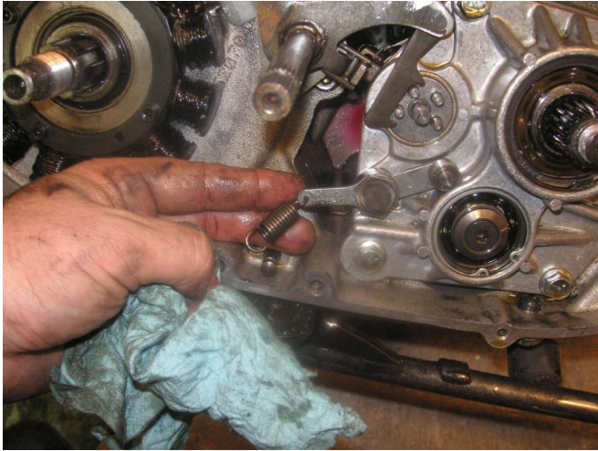
When the clip and drum popped off the shift drum, the spring came off the case mount.
