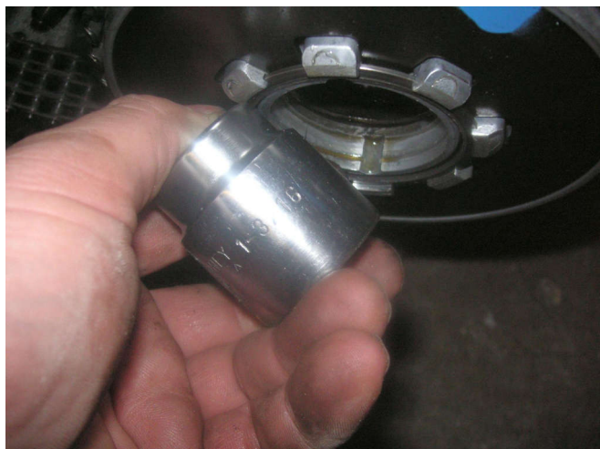
It's an inch-3/16 socket to get the clutch basket off.
