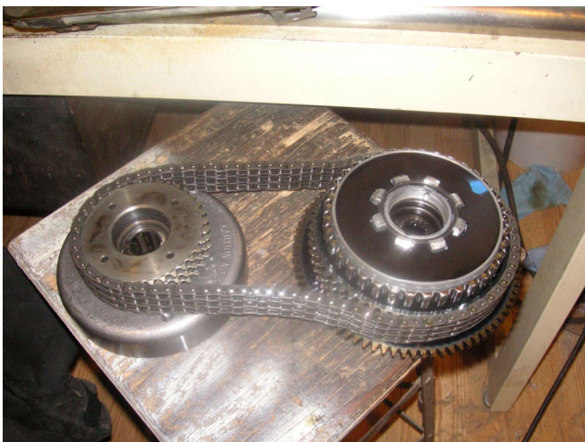
Here is the primary off the bike. Magnetism resists the alternator rotor coming off.
