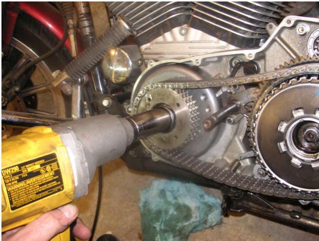
I have an old DeWalt corded impact wrench that gets the nuts off no problem.
