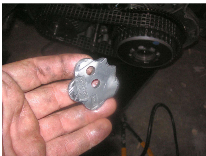
This is the detent drum that holds the bike in any given gear. It fell off with the clip.
