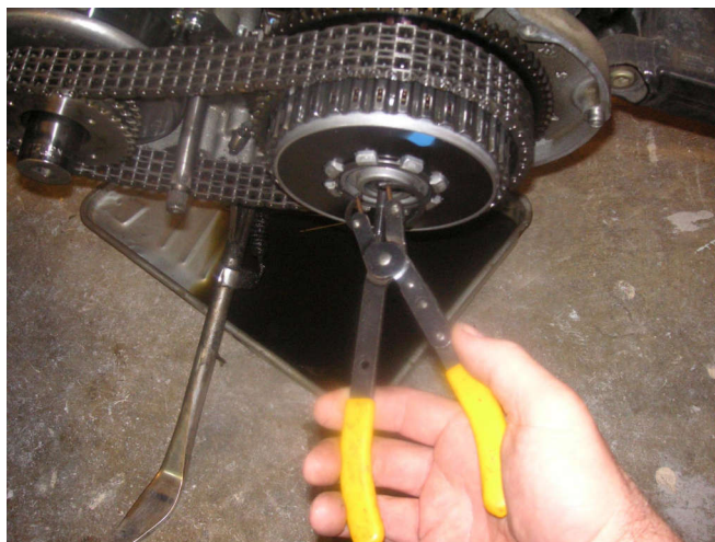
I remove a snap ring from the clutch basket. I wished the shift drum used one as good.
