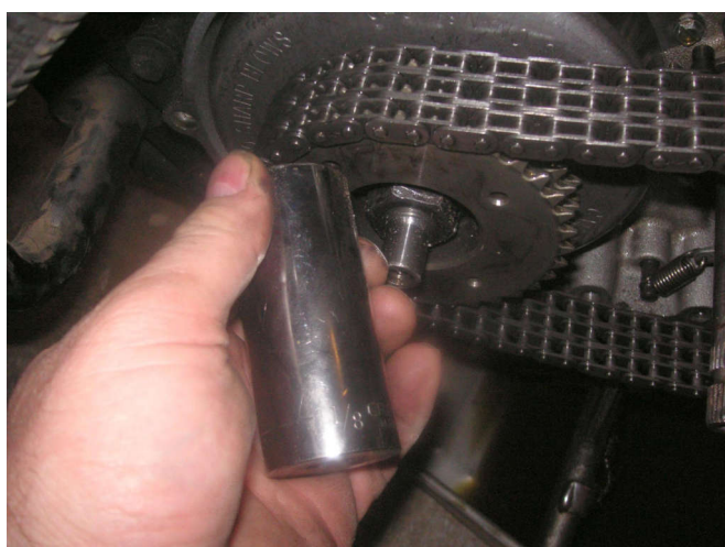
The deep-well 1-1/8 socket gets past the sprocket shaft and pulls the nut up front.
