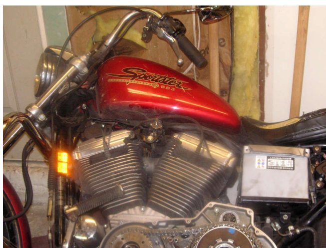
Leaned over, it's a lot easier to work on with the primary leaned up towards you.
