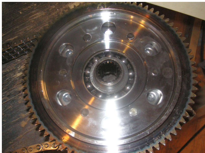
I was worried the loose detent drum had torn up the back of the clutch basket. Lucky me, the clutch basket was OK, no collateral damage.
