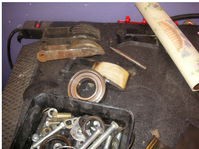
I also replaced the trap door bearing and the chain tensioner and its spring.
