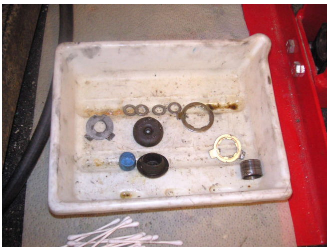
Three lock-washers, the ruined countershaft bearing, and a couple plugs are left over.
