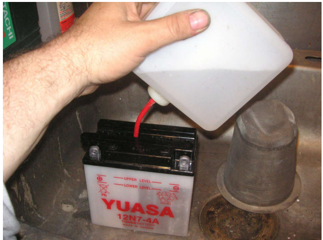
I learned it is best to just put a new battery in any bike that has sat for more than a year. Here I add the acid. I like Yuasa brand batteries.
