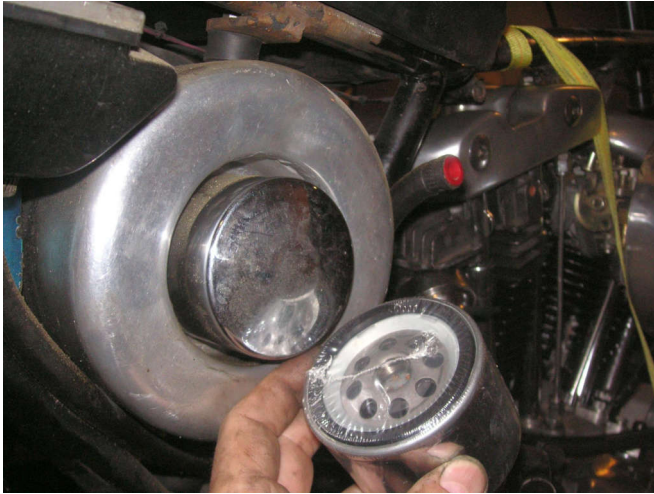
I change the engine oil and filter. The oil is full of aluminum particles from the blown piston.
