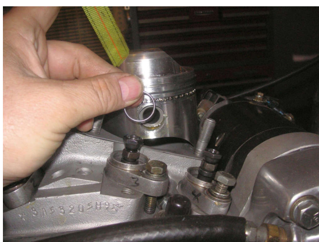
You put the pistons on the rods and clip in the piston pin.
