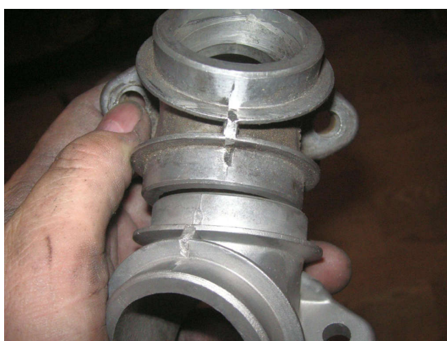
Note the big divots in the intake manifold. This can be a killer air leak.
