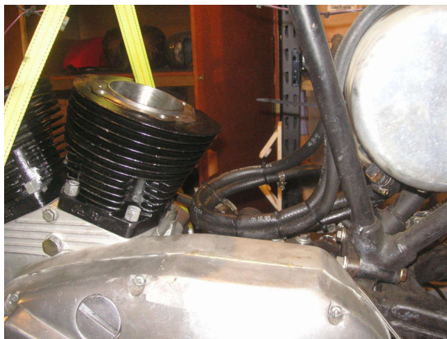
The cylinders are on, I made sure to wash them before oiling them up.
