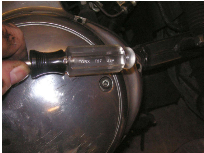
A Torx T27 for the derby cover. I hate Torx even more than Allen heads.
