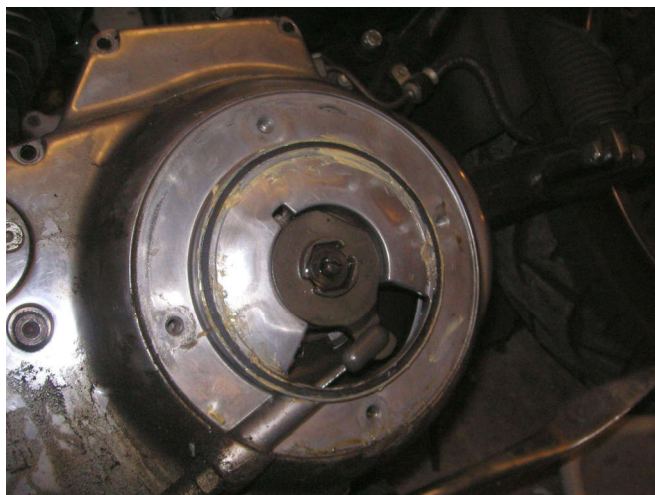
The clutch mechanism is revealed. It is a really nice pressed-metal piece, not like an Iron Sport.
