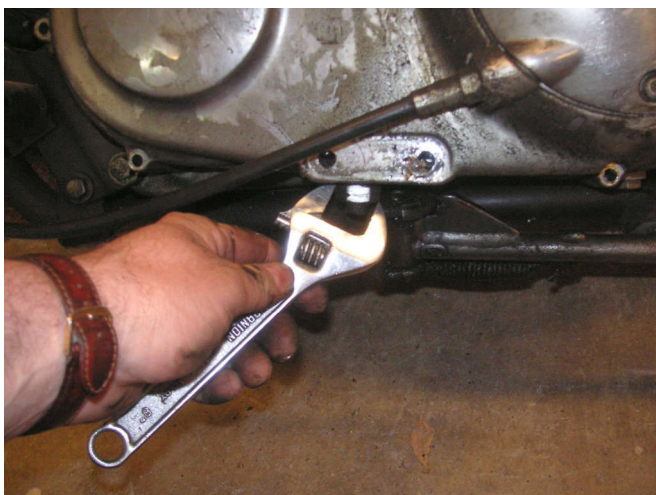
This is the tensioner nut and bolt for the primary chain. Back it way out.
