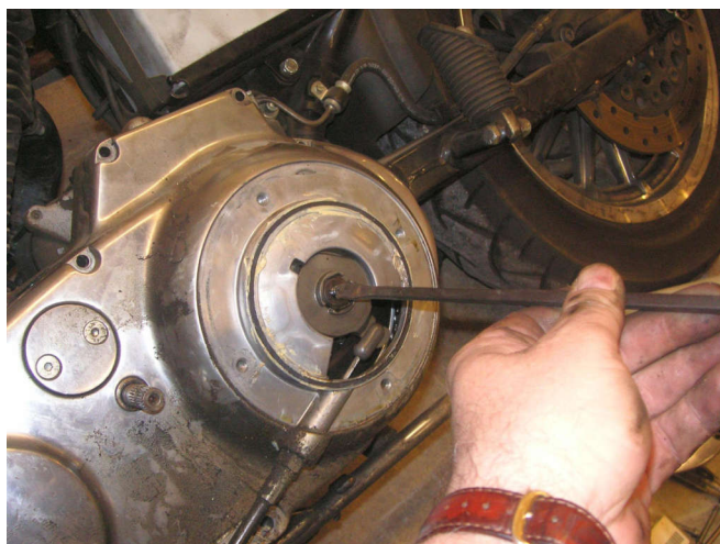
Back out the screw and that lets the captivated nut come out of the mechanism.
