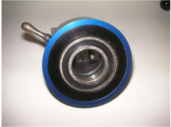
This is where the cutters fit. It has a precision bearing for the cutters to spin on.
