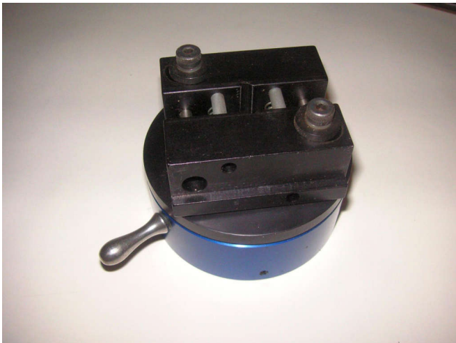
Here is the clamp mechanism for the valve stem. This sold fast on eBay, I can't remember what I got for it..
