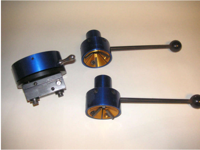
I had two different angle cutters. They fit into the unit at left, which clamps the valve stem.
