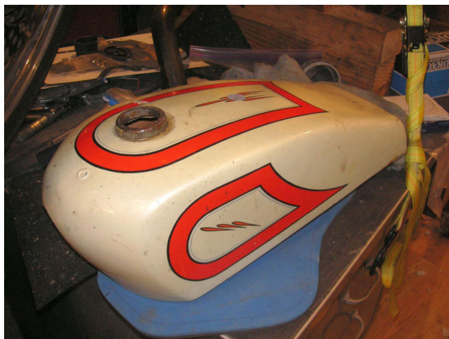
The tank developed pinhole leaks so I had to toss it out.
