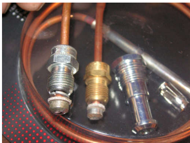
I noted the spring washer on the old unit to keep pressure on the pill. New stuff is cheap.
