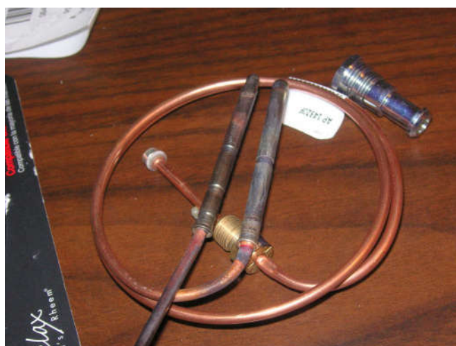
The old unit did not have a lot of carbon on it. Sanding it clean did not get it working. These must fail a lot if Home Depot has them in stock.
