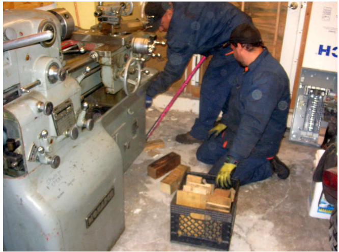
The fork truck would not fit in the garage, so the guys started to block up the lathe.
