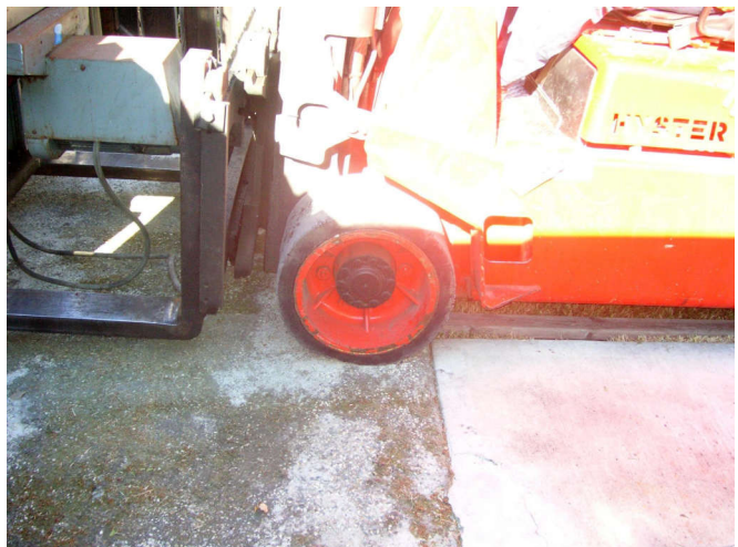
One problem was the X-axis motor that stuck out so far it put the machine on the tips of the fork. They put cribbing under the tires.
