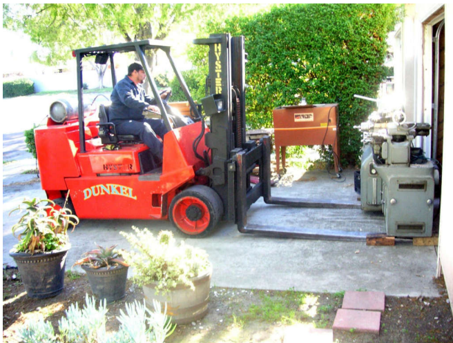
Good riggers with good machinery. They slip the forks under the lathe.
