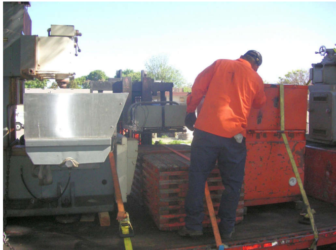
The riggers check that everything is strapped down.
