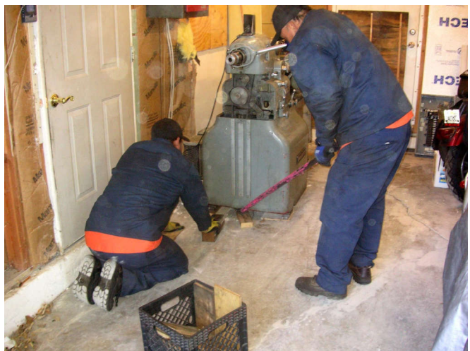
They needed to get the lathe high enough to get a pallet jack underneath it.
