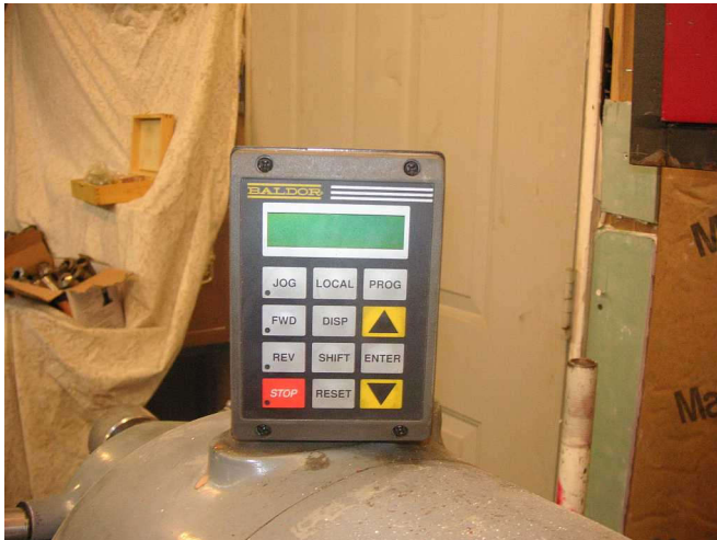
This inverter gives the lathe fingertip-adjustable speed without having to change gears.
