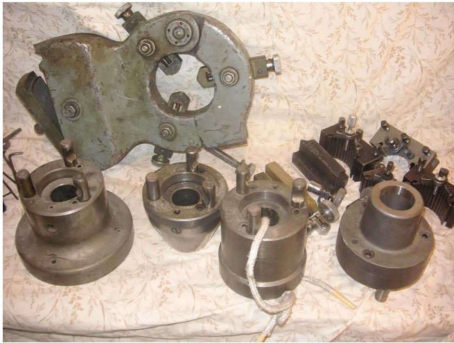
A steady-rest and more special chucks came with the machine. I kept it all together..
