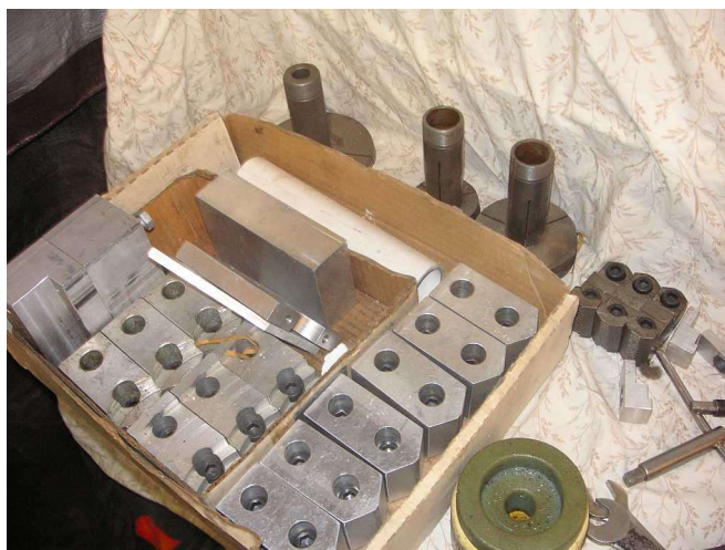
The lathe came will all these soft-jaws. More stuff that is worth a lot all by itself.
