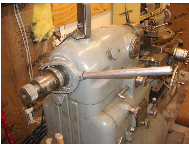
There was a collet changer on the machine. It was used to make RF wave-guide parts.
