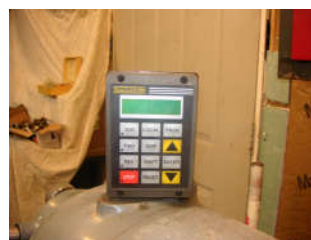
Lathe had a flux-vector speed control.
