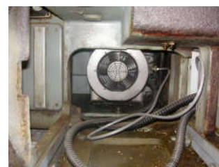
Lathe had a flux-vector speed control.
