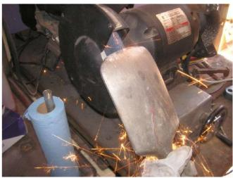
The jackhammer came with a spade bit. Since I had to cut through roots I sharpened up the bit.
