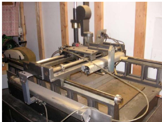
The back view shows the X-axis linear optical scale.
