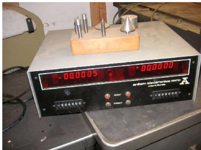
The CMM had an Anilam readout.
