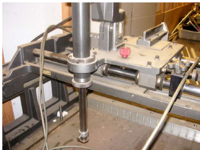
The Z-axis drops down so a cone can center on whatever hole I needed to measure.
