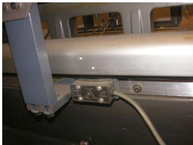
There were two linear optical scales. The unit was not as accurate as an air-bearing CMM, but it did the job I needed it to.
