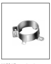
NACC VR mounting clamps may be used to mount any cylindrical capacitor with a 1" to 3" diameter that is to be mounted in a vertical position. Material is 1010 CRS, commercial grade #4 temper ASI-scale. Parts are finished with .0001 (nominal) zinc chromate plating. Use for mounting CG types, PSU, HC/NP and MPD/MPF types. Material thickness is .035"
