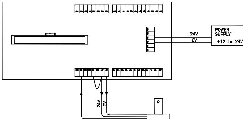
Depending on the output of the flag, the return line (RETn) to the ACC-8F could be wired to the flag power or ground.
