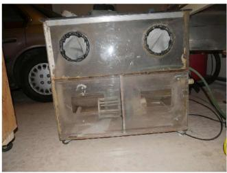
You can see the shop vac in the bottom chamber. I also put a big shop vac on the vent outlet. This keep the beads from going all over.
