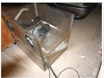
This end has the air in, vent out, and electric.
