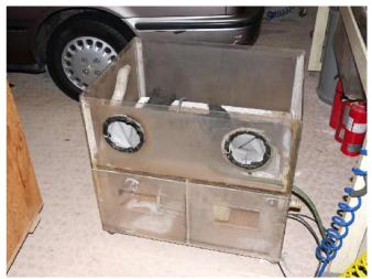
The cabinet top lifts off to add beads and put the parts inside. Three is a deck built with screen-door screen so the beads drain down. The square holes are for clean-outs.
