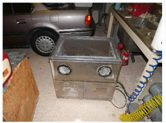
Ready for use with the top on. I had to increase the top plastic to 3/8 inch. It would flex under vacuum and break the glass glued on underside.
