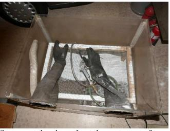
Sto mount the gloves I cut the center out of two one-gallon can lids. They press into holes.
