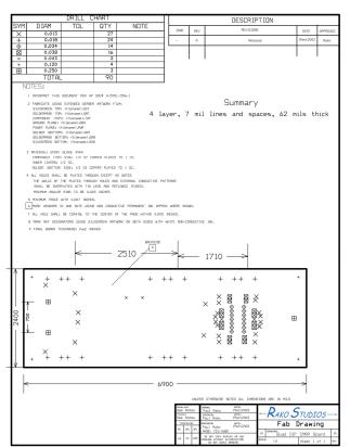
This board mounts SMA connectors that screw directly into an HP3577A network analyzer. This removes any effect from cables. The BOM (pdfs in design files).
